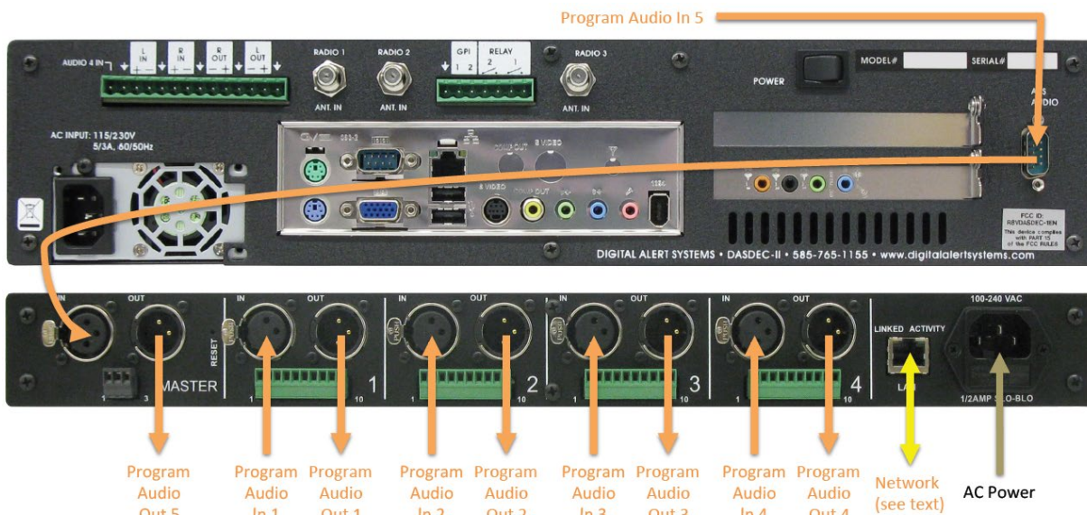
Figure 6 DASDEC and MultiPlayer audio program wiring configuration
